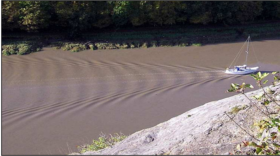
Figure 7: Deep water ship wave pattern. (Photograph by Adrian Pingstone)
