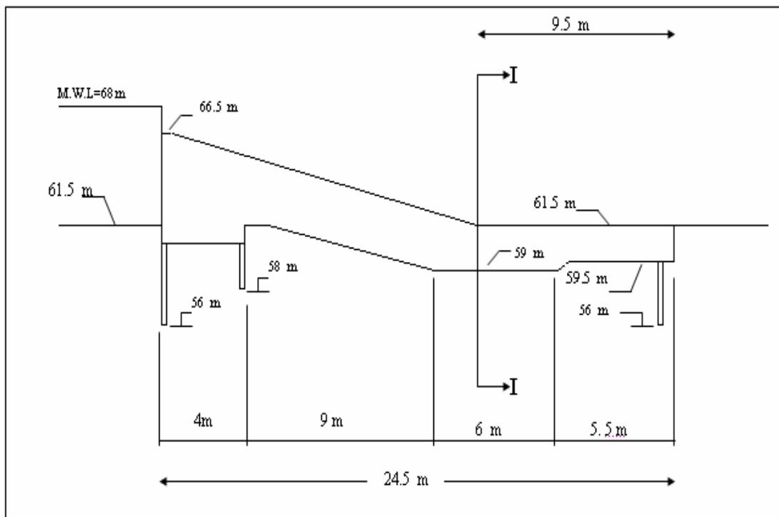
Fig. 2: Dimensions of Diyala Weir Structure
