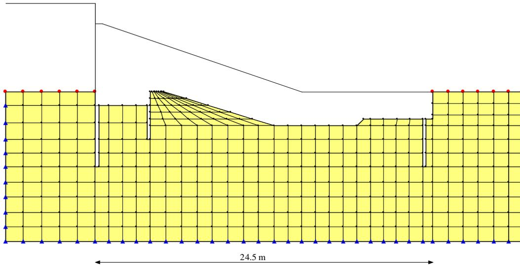
**Fig. 3: Finite element mesh for Diyala Weir resting on pervious soil foundation**
