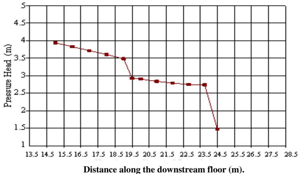
**Fig. 5: The total pressure head distribution underneath Diyala Weir floor along the downstream apron**
