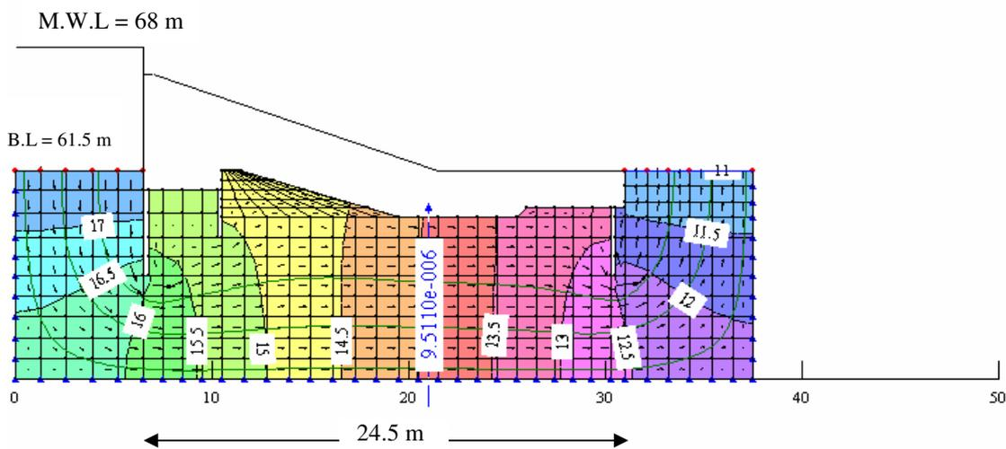
**Fig. 4: Seepage of water underneath Diyala Weir Foundation**
