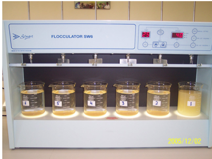
Figure 3. Jar test for high turbidity river water
