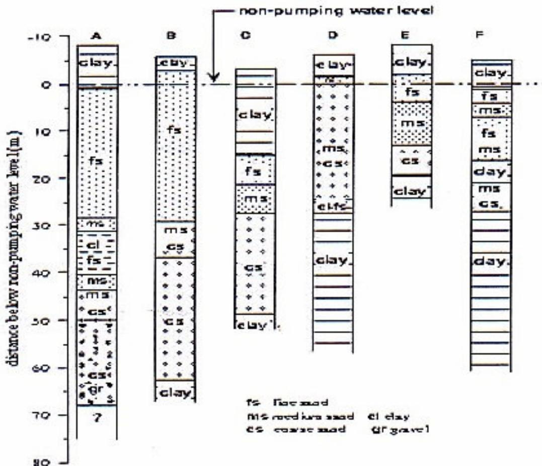
Fig. 2 Strata of six bore logs
