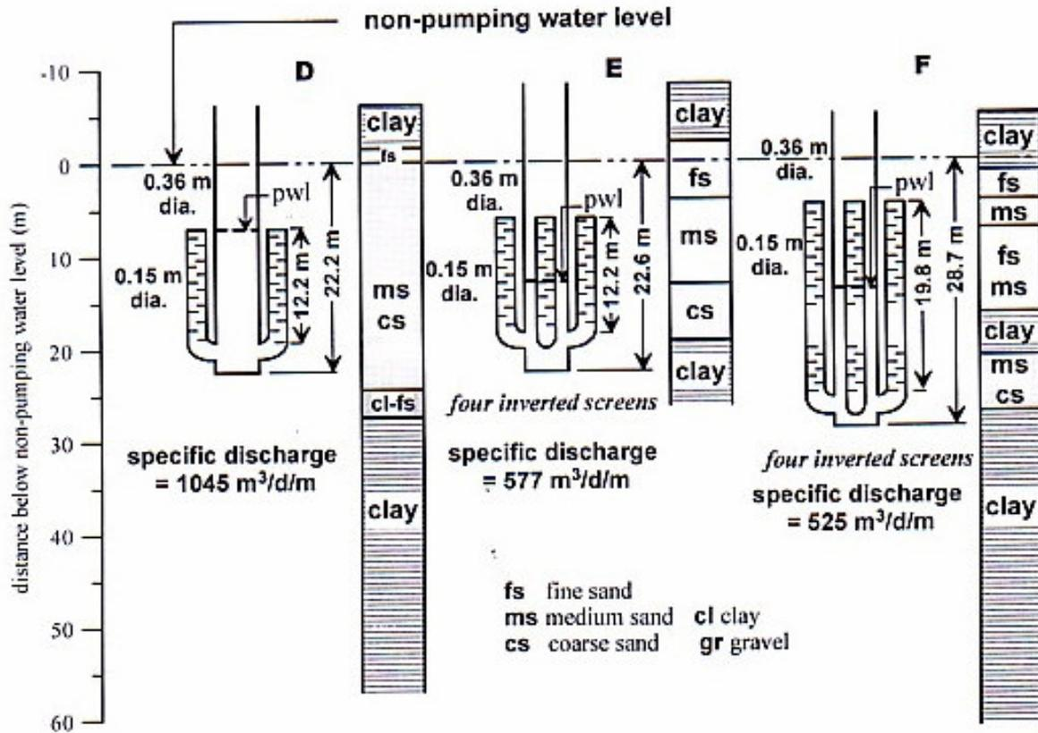
Fig. 4 Inverted wells at locations D, E and F.
