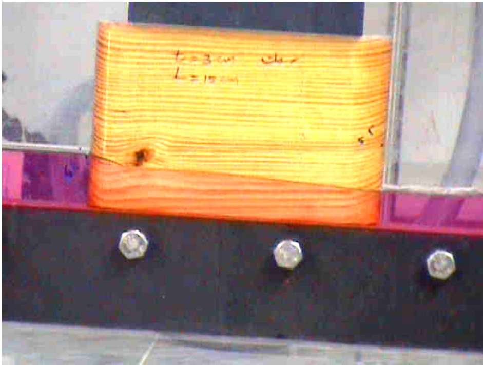
Photo 1 Backwater rise due to subcritical flow condition between piers.
