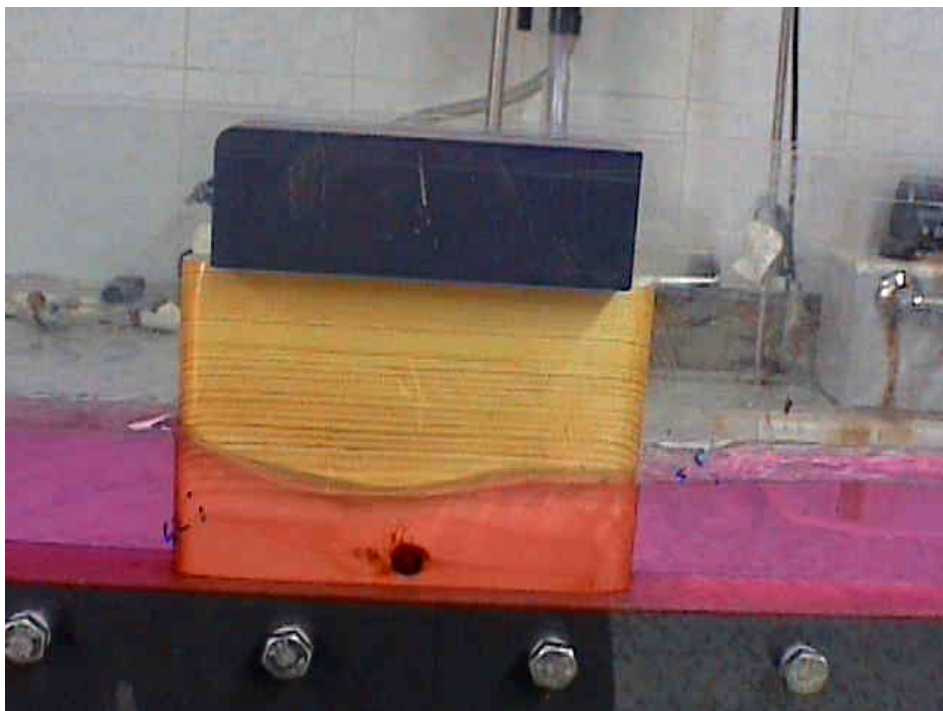
Photo 2 Backwater rise due to supercritical flow condition between piers.
