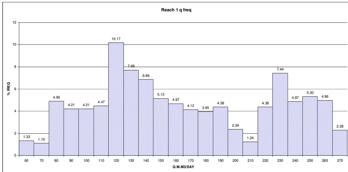
**Figure 1. D.S. Aswan Dam discharge Frequency distribution**
