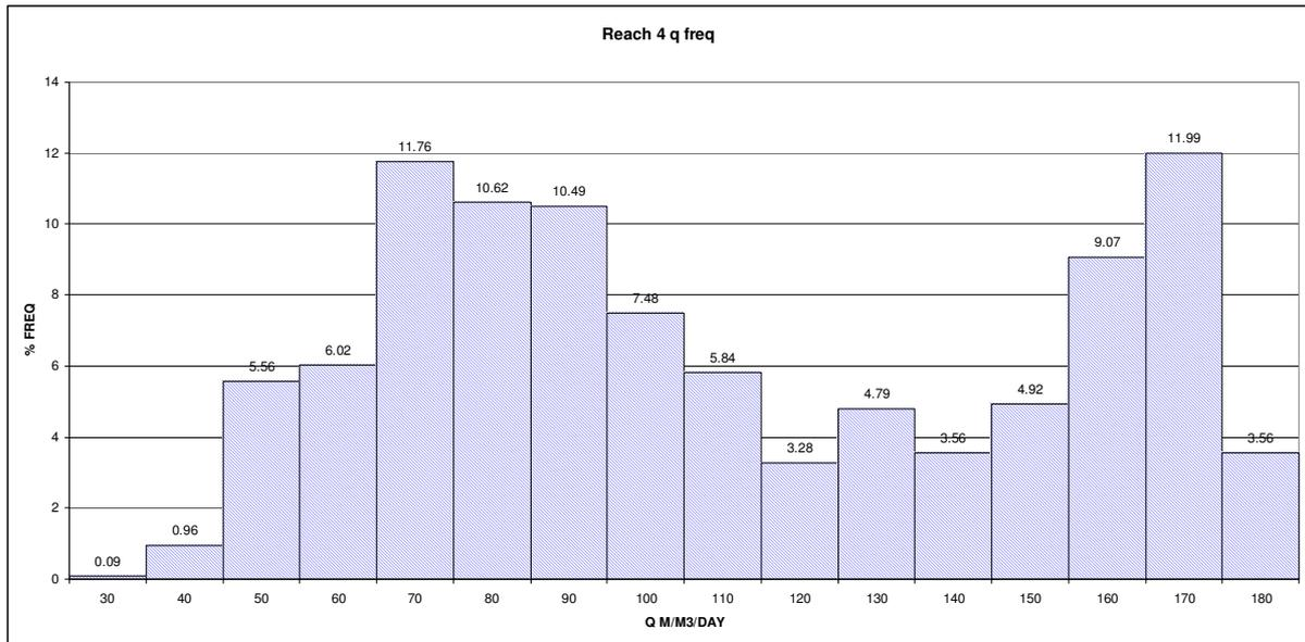
Figure 2. D.S. Assiut Barrages discharge Frequency distribution
