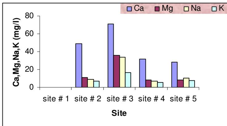
Figure (8) Calcium, Magnesium, Sodium and Potassium of the water samples from different sites the study area
