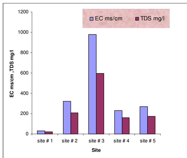
**Figure (6) TDS and Electric Conductivity of the water samples from different sites in the study area**
