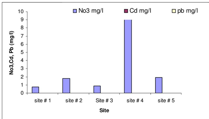
**Figure (10) Nitrate, Cadmium and lead of the water samples from different sites the study area**
