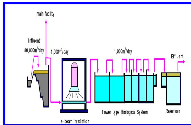
Fig. 2 Schematic of the pilot water treatment plant in Daegu, South Korea, [5]
