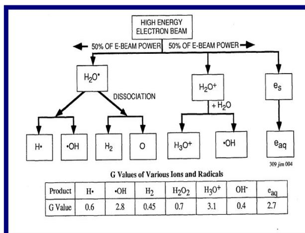
**Fig. 1 Various ions and radicals formed by electron beam irradiation of water. The G value is defined as the number of species produced for every 100 eV of electron beam energy absorbed [1]**
