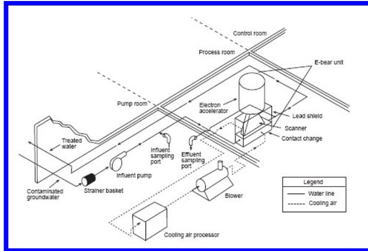
Fig. 3 Schematic of the HVEA E-beam treatment system, [6]
