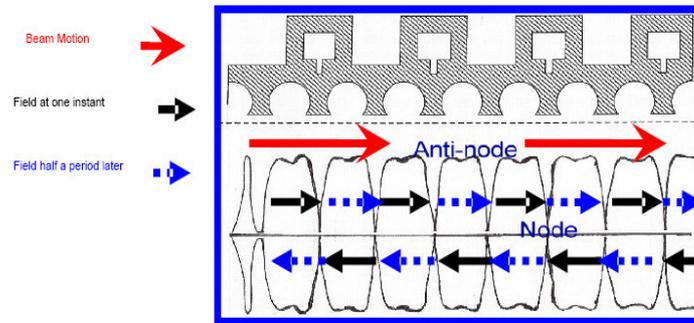
**Fig.5. A standing wave pattern in a linac**
