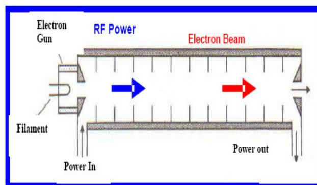
Fig. 4. Schematic of a traveling-wave linac, [7]
