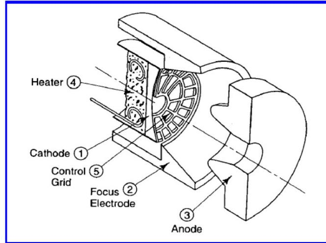
**Fig. 7. Schematic cutaway view of a triode thermionic electron gun, [8]**
