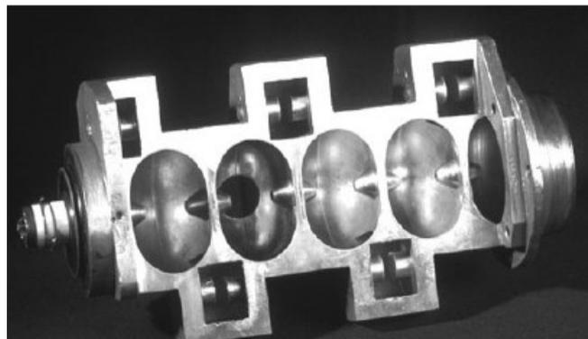
**Fig. 6. Cutaway view of a standing wave accelerating linac. The cavities are clearly visible: the accelerating cavities are on the central axis; the coupling cavities are off-side, [8]**
