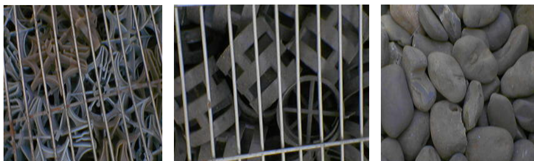
Photo (1) the three used media (Star shape, pall rings and gravel) respectively
