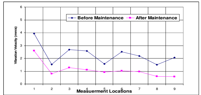
Figure (9) Overall vibration level before and after maintenance for unit (6)
