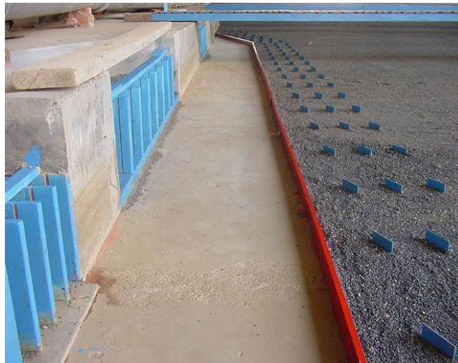
Photo 2 The arrangement of the Tested Submerged Sill and Bottom Vanes in the Model
