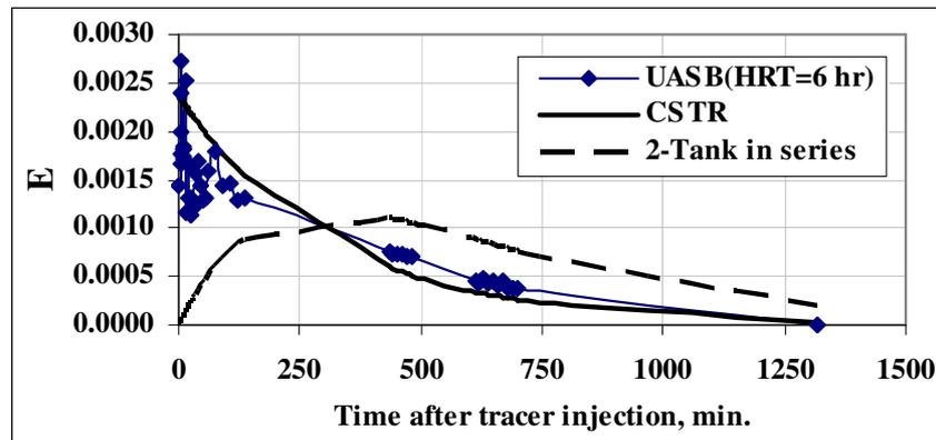
**Figure (9) Dimensionless E curves for the UASB, CSTR, and 2-tanks in series (at 6 hr-HRT)**
