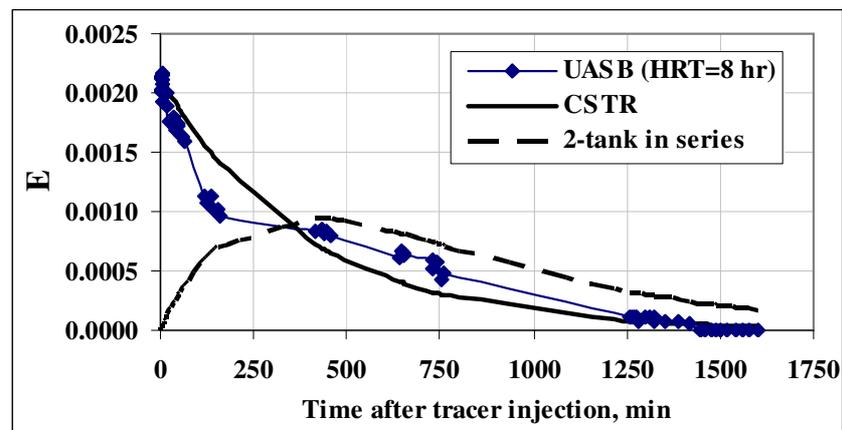
**Figure (10) Dimensionless E curves for the UASB, CSTR, and 2-tanks in series (at 8 hr-HRT)**
