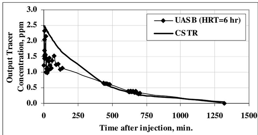
Figure (6): Output tracer concentration vs. time for the UASB reactor and CSTR (at 6 hr-HRT)
