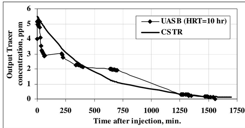
**Figure (8): Output tracer concentration vs. time for the UASB reactor and CSTR (at 10 hr-HRT)**
