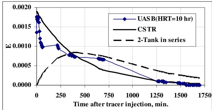
**Figure (11) Dimensionless E curves for the UASB, CSTR, and 2-tanks in series (at 10 hr-HRT)**
