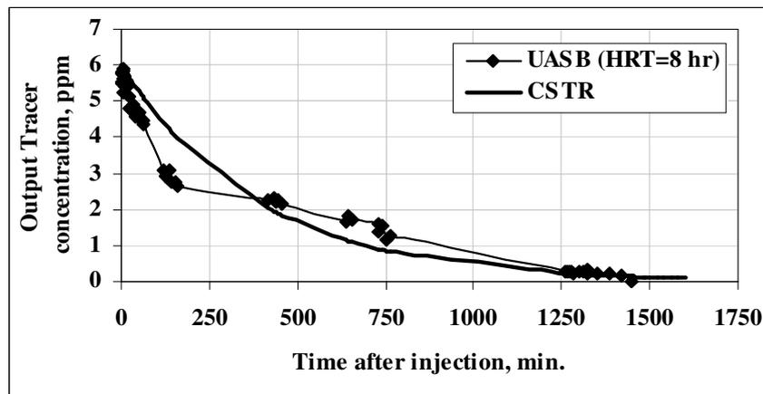
Figure (7): Output tracer concentration vs. time for the UASB reactor and CSTR (at 8 hr-HRT)
