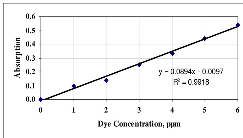
**Figure (2): Tracer Calibration Curve**
