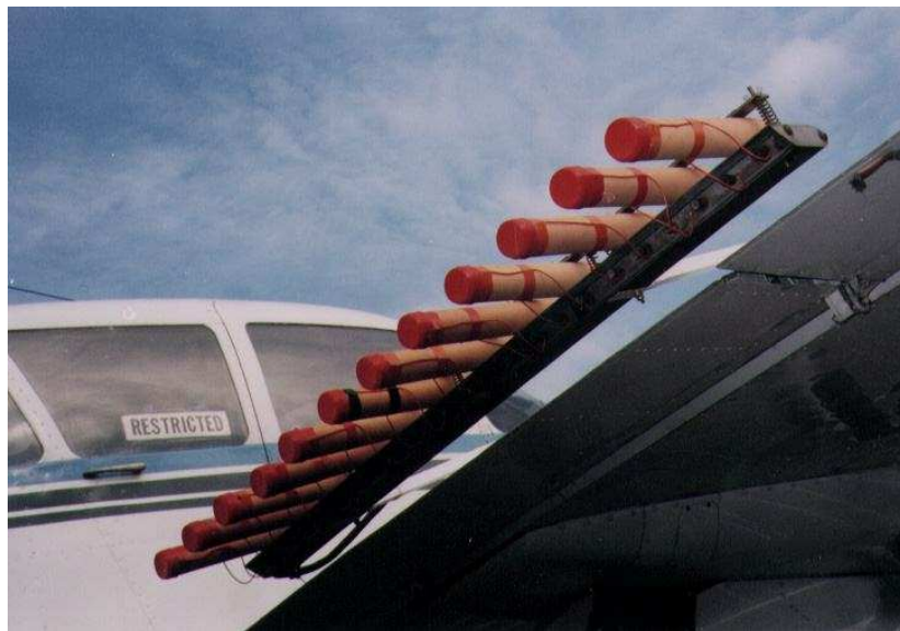
Figure (2) Fixing Silver Iodide Bombs in the Aircraft
