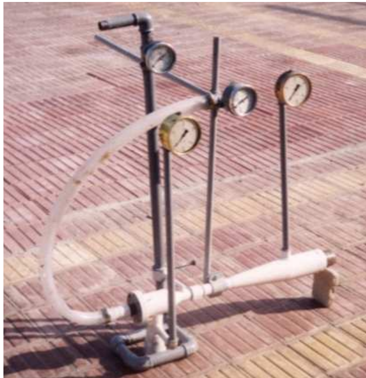
Fig. (2). Photo of jet pump and fluidizer used in experimental test rig
