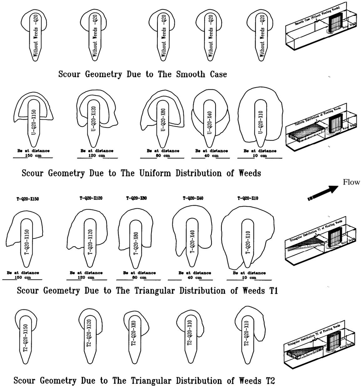
Figure (2) Scour Geometry for Different Distributions of Floating Weeds
