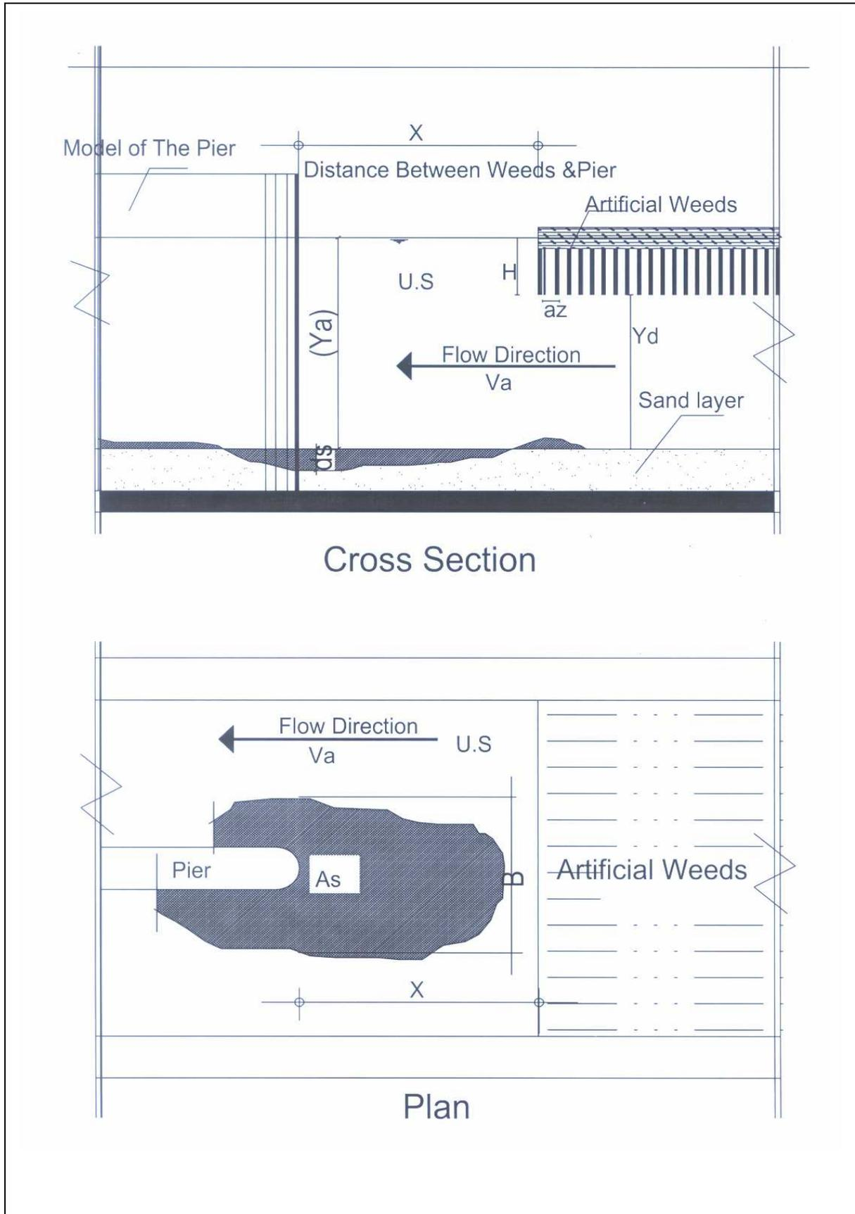
Figure (1) Definition Sketch Showing Dimensional Analysis Parameters
