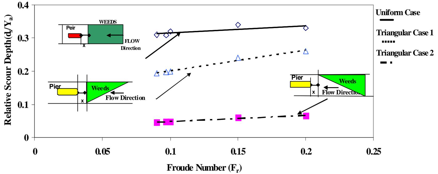
Figure (4): The Relation between Froude No. and Scour Depth for Different Distributions of Floating Weeds
