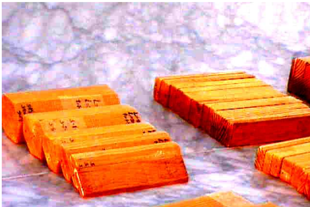
Photo 1 The rectangular and triangular pier models
