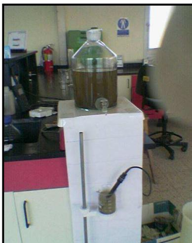
**Figure 4: Arrangement utilized in measuring DO conc. at different heights**
