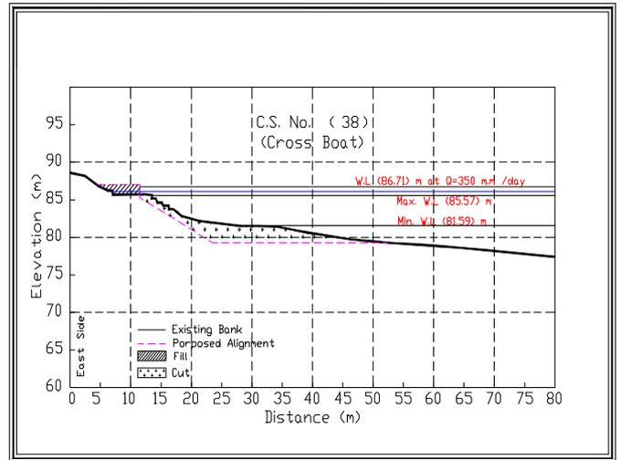
**Fig 5 Proposed Modification of the Berths Cross Sections**
