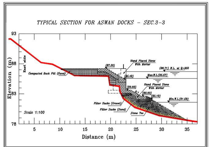
**Fig 6 Typical New Proposed Berths Design**
