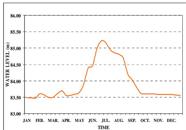
**Fig 3 Typical Water Level Hydrograph at Aswan Station**
