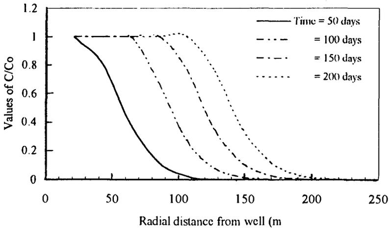
Fig. 7 Relative concentration  $C/C_0$  versus radial distance from well with time for  $k = 50$  day,  $T = 100$  m<sup>2</sup>/day and  $T_s = 2000$
