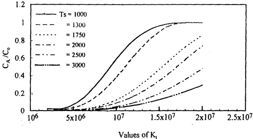
Fig. 10  $C_A/C_0$  versus  $K_1$  for various values of  $T_s$  (for 3 wells)
