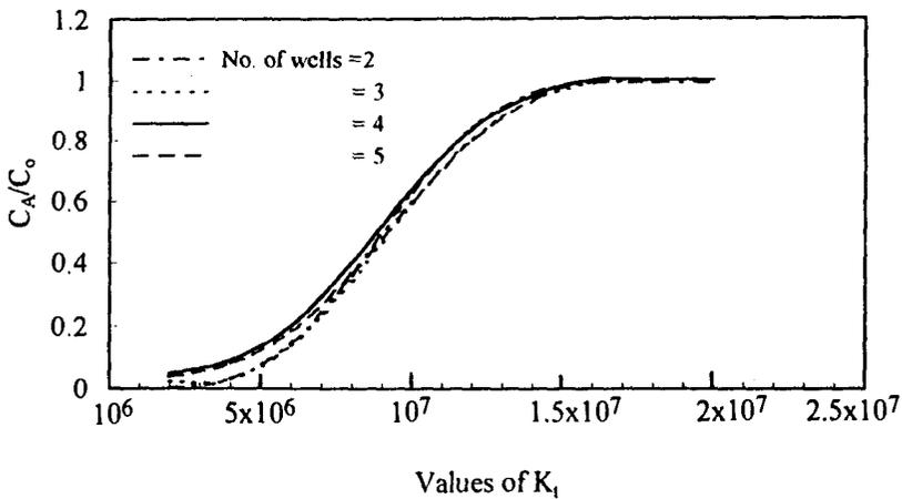
Fig. 11  $C_A/C_0$  versus  $K_1$  for different No. of wells at  $T_s = 1000$
