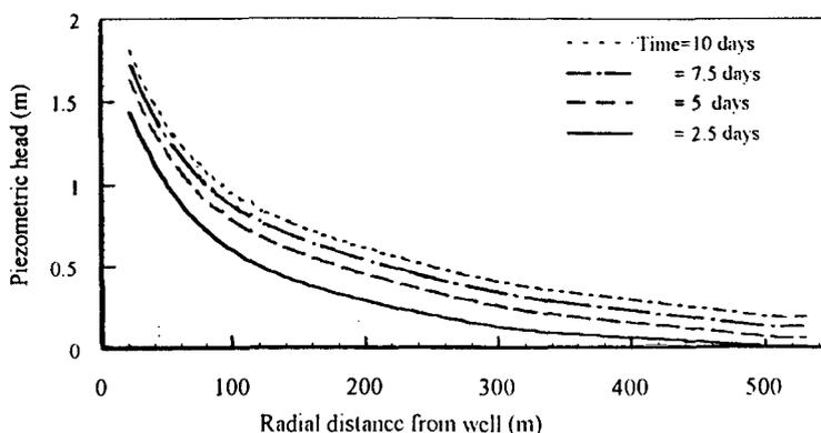
Fig. 5 Piezometric head ( $h$ ) versus radial distance ( $r$ ) for different Times
