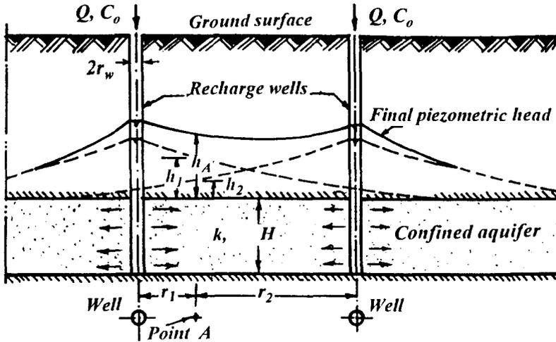
Fig. 3 Multiple recharge wells in confined aquifer.
