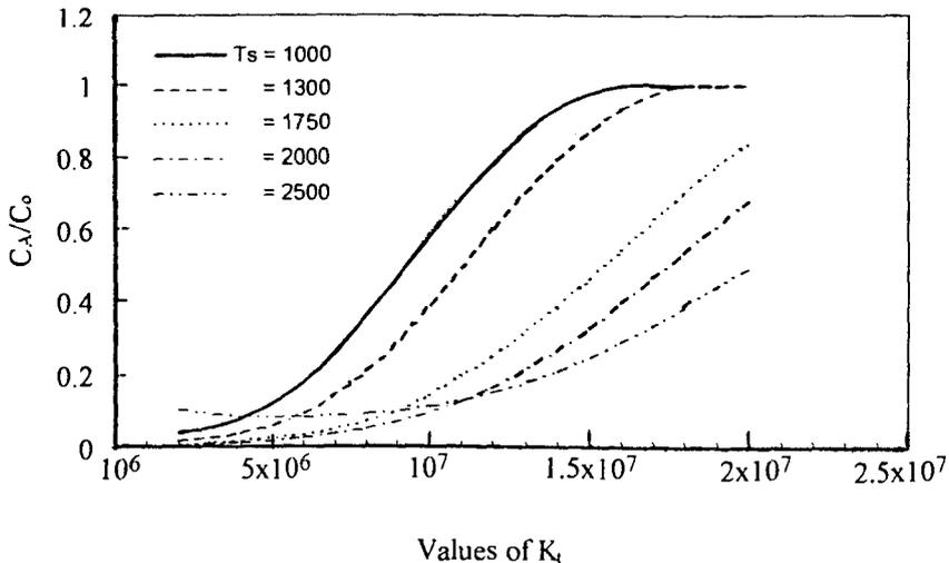
Fig. 9  $C_A/C_0$  versus  $K_t$  for various values of  $T_s$  for 5 wells.
