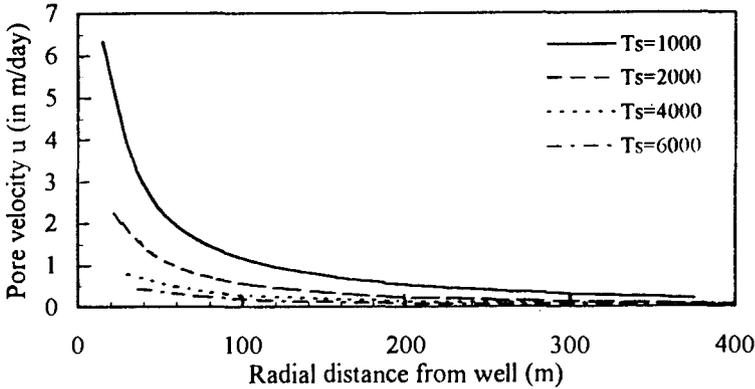
Fig. 6 Pore velocity ( $U$ ) versus radial distance ( $r$ ) for different  $T_s$  values,  $k = 50$  m/day and  $K_1 = 5 \times 10^6$ .
