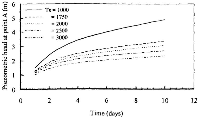
Fig. 8 Piezometric head at A versus time for different values of  $T_s$  ( $k = 100$  m/day,  $d_s = 1.00$  mm,  $\phi = 0.4$  and  $S = 0.004$ ).
