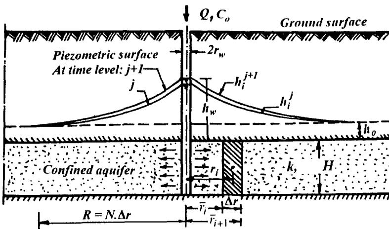
Fig. 1 Radial flow from recharge well in confined aquifer.
