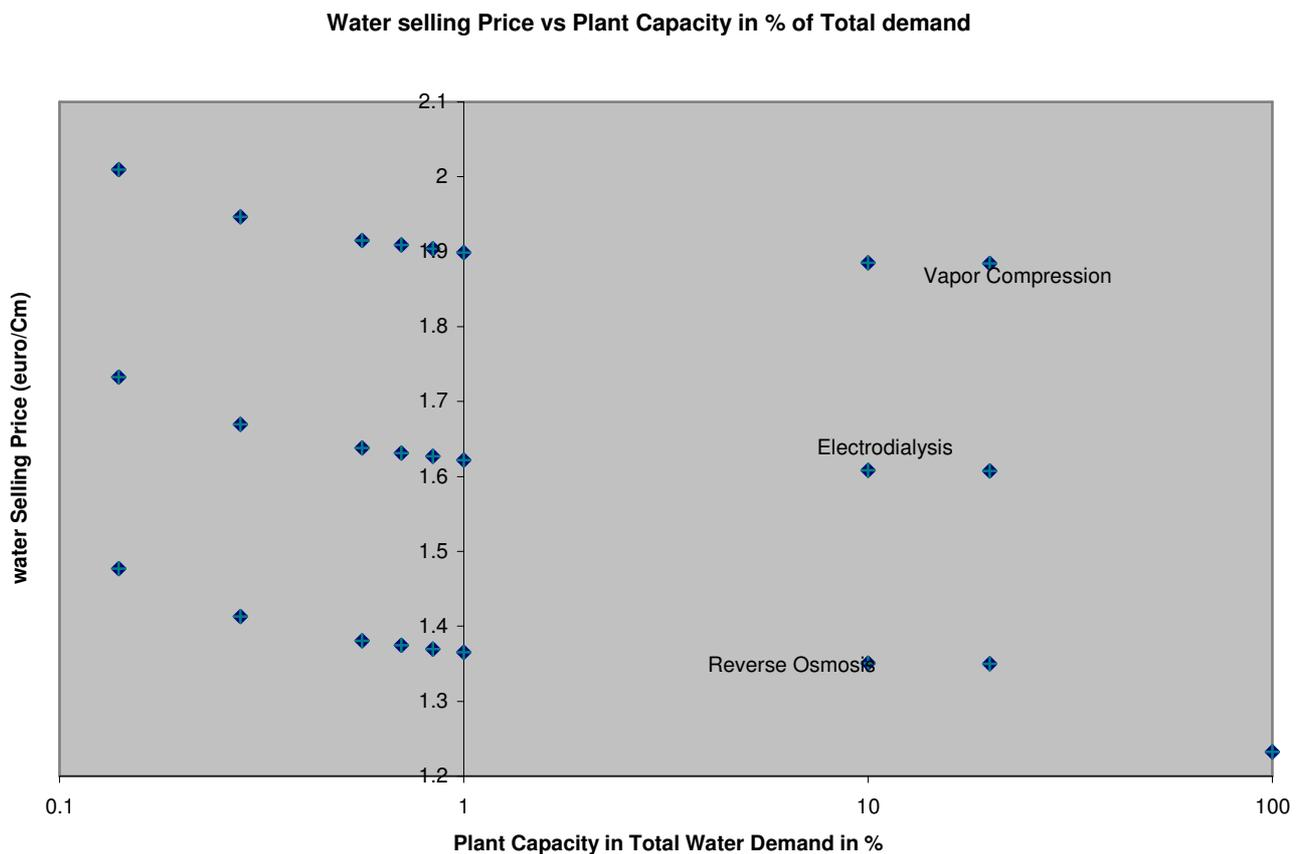
**Figure 3: Selling prices of desalinated water versus desalination plant capacity**
