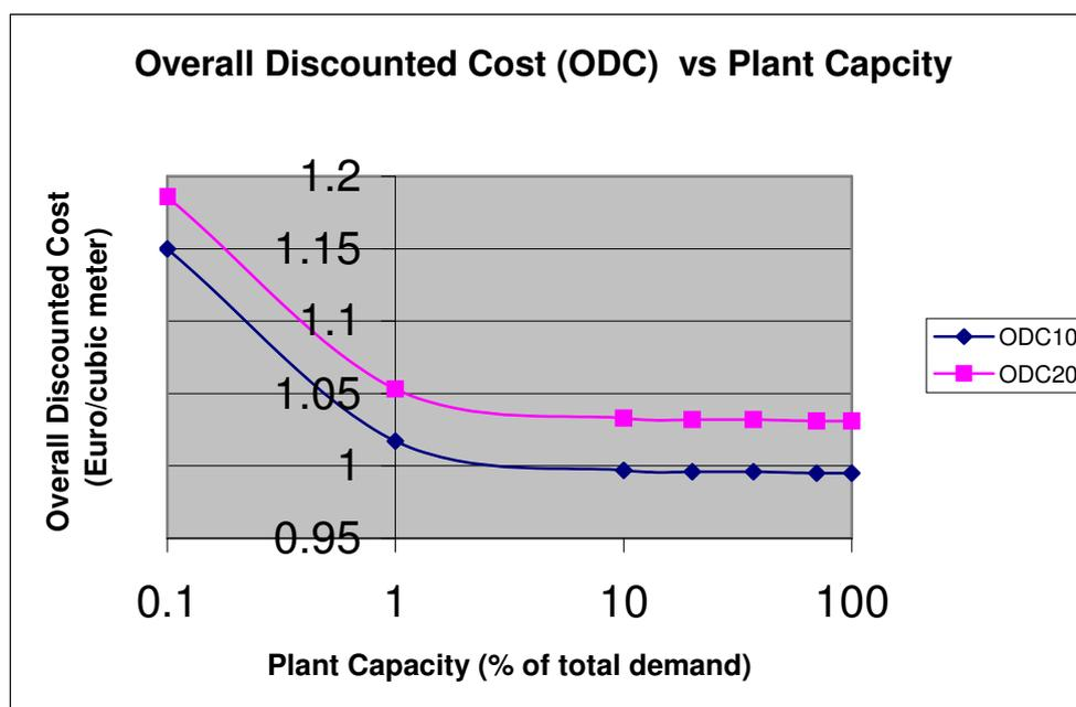
**Figure 4: Overall discounted cost of reverse osmosis desalination versus plant capacity expressed in percentage of the total demand (120 mcm) for two coverage percentages of the energy needs by photovoltaics (10%-ODC10 and 20%-ODC20%)**
