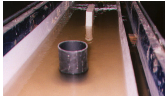
Photo (3) Scour holes around circular pier in U.S. with Rect. pier in D.S.
