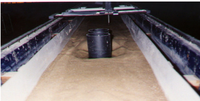
Photo (1) Scour holes around two circular Piers
