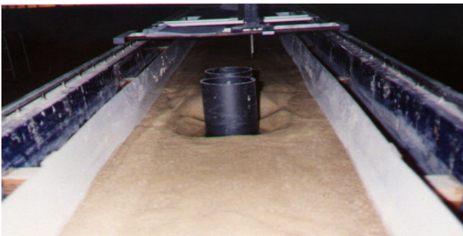
Photo (1) Scour holes around two circular Piers
