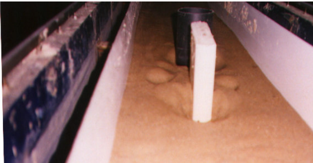
Photo (2) Scour holes around rectangular pier in U.S. with circular pier in D.S.
